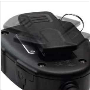
Clothing clip. 360° Rotation with positive detent stop every 45°
