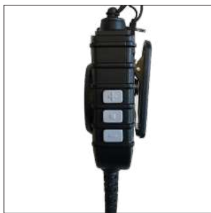
Volume +/- buttons and loudspeaker on/off switch when headset connected.
